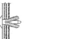
Remove dust and filings from the hole. Insert rivet.
