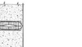
Rivet expands into hole turring steps studs, squares of brick block, concrete, drywall
