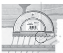
Example of properly troweled adhesive application
